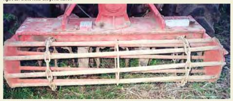
Note the crumb roller at the back of the harrow. You can just lower the roller part if you want to break up clods on the surface of the soil without disturbing the soil underneath.
