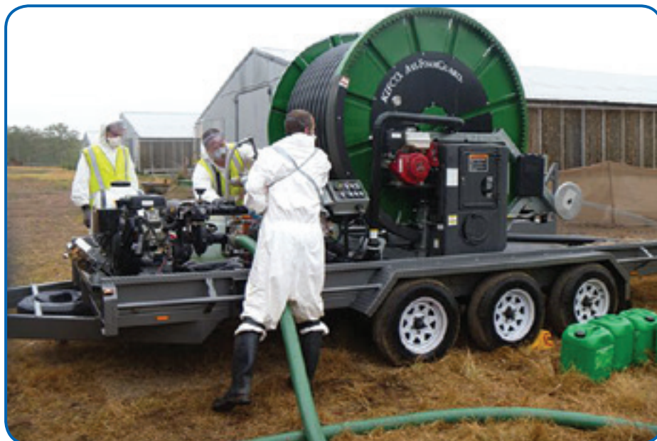
Poultry in the sheds where H7N7 avian influenza occurred were humanely euthanased by using a foaming machine. Photo by K Cooper
