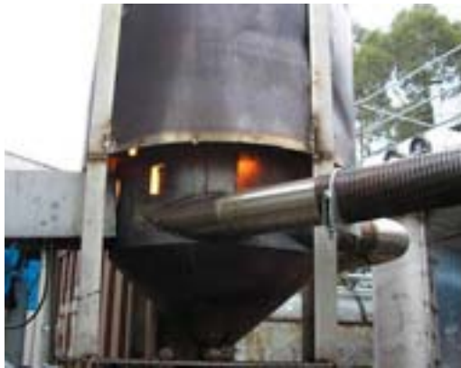
A pilot biochar reactor in Gosford
