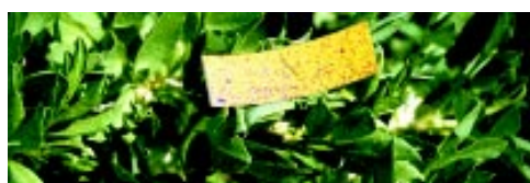
Litmus paper can be used to assess spray coverage throughout the canopy
