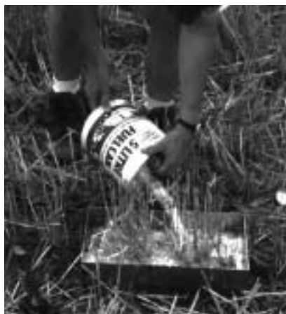
Figure C4-5. Pouring a white paint solution into a soil to assess the presence of continuous vertical macropores.
