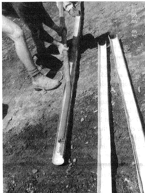
Extruding an ASS core from QASSIT'S vibro-suction corer.
