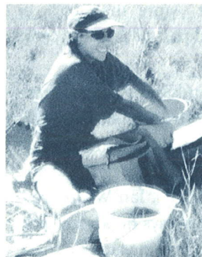
Kylie Hey Qld's ASS Information Officer conducts a field peroxide test at a spoon-drain (less than 30cm deep) for Maroochy Council's mosquito control program.
