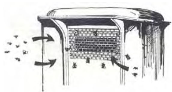
Mesh excluder fitted to bait bin fly trap
