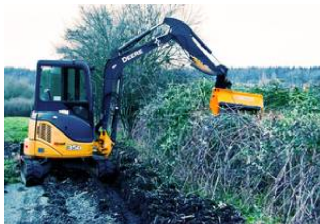
Above: An excavator mounted flail mower is used to mow down and mulch a high and potentially inaccessible thicket to the ground.
