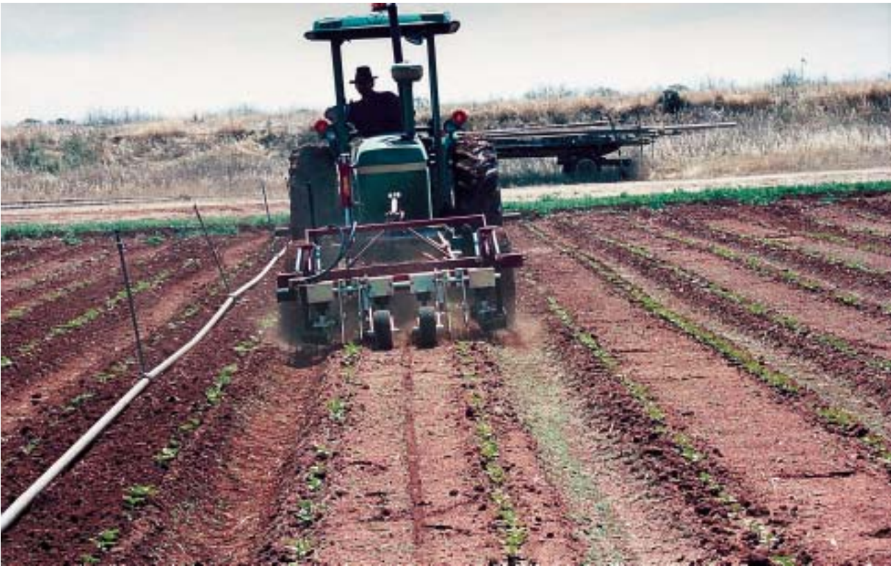
The Weedfix® cultivator is an effective implement for controlling post-emergent weeds in crop rows. It is a cultivation machine consisting of a series of rotating tines that remove young weeds through a ‘stirring’ action on either side of the crop row. Crop guards, mounted adjacent to the tines, protect the crop from damage.
