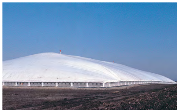
Figure 2. Experimental use of CO 2 in a maize bunker, Peoria, USA. Photo HJ Banks (© CSIRO)
